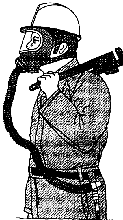
Figure 1-31.—Supplied-air respirator hose-line mask.
