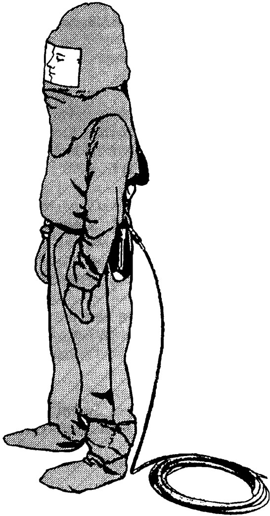
Figure 1-32.—Disposable spray-painting hood.
